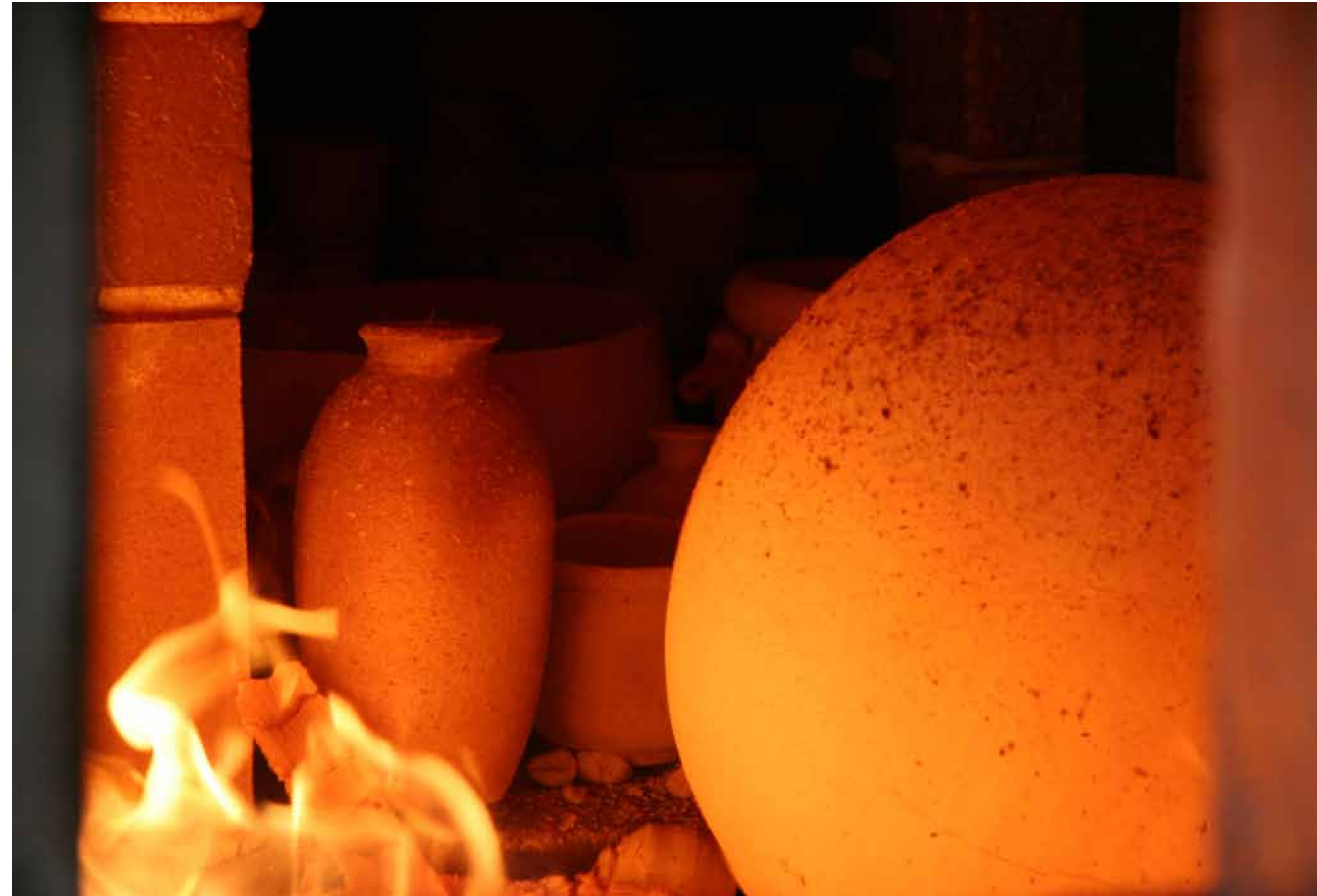
A quick look: The interior of the kiln at about 800°C. The ash particles on the ceramics are clearly visible
